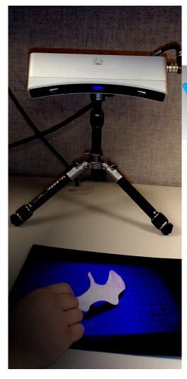
Ian Sayers, Peak Solutions LLC, rapidly scans the fossil casts using the Geomagic Capture scanner into Geomagic Wrap for fast preparation into watertight 3D models for printing.
