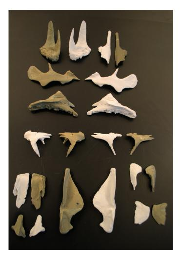
"The ProJet 660 produces hardened gypsum parts and this is an ideal surface to paint on," said Holland. "We usually use the full-color features of these printers but this time we went for monochrome prints so we could add realistic finishes. The ProJet 660 parts are rigid and bone-like and also work well with the glue, pins and nails that we use for constructing skeletons, so it was a perfect choice."
